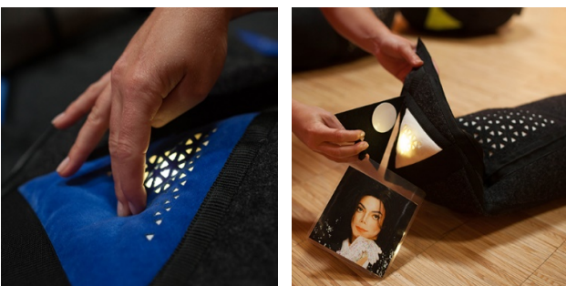
Figure 2 & 3: Soft and sensorial stimulating Touch- and RFID-sensors with light response. © Birgitta Cappelen
